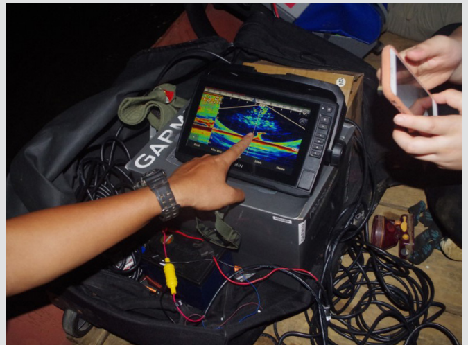
This machine uses sound waves to detect irregular objects (e.g. a large turtle) under the surface. Photo credit: Jack Carney (ATP/IMC)
